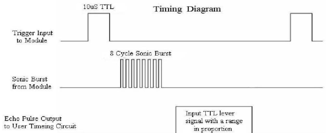
To use with an Arduino, the Arduino is used to generate a 10 $\mu$ s pulse on the trigger pin of the SR04 to start distance measurement.
